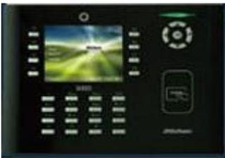
The device supports up to 50,000 users and 150,000 event log registrations. The system connects to an existing computer network or directly to a computer over the network (UTP) cable. Device is designed for indoor or outdoor (with use of special housing) mounting.
