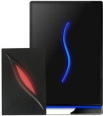
The device supports up to 10,000 users and 30,000 event log registrations. The system connects to an existing computer network or directly to a computer over the network (UTP) cable. It is designed for indoor or outdoor mounting. It has simple use and enables fast employee flow.
