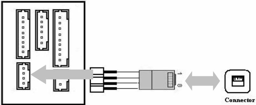
1).TFT screen Fingerprint Machine connects with PC through cross cable
