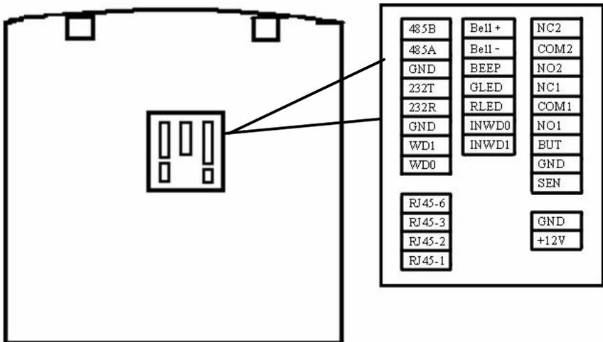
Table 1 the definition of the Pin of TFT screen Fingerprint Machine connector
